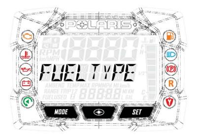
When using the recommended 91 non-ethanol gasoline, always select the 91 NON-ETHANOL setting. When using ethanol, MTBE, or other forms of oxygenated gasoline, the fuel type must be changed to NON-PREMIUM/ETHANOL in the gauge.
