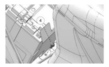
8. Remove the battery shield ⑤.
