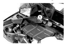
3. Disconnect the hood wire harness connector ②.
