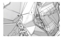
3. Remove the plastic rivet ② securing the fender to the chassis.
