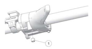
2. Move the control block to the desired position.
