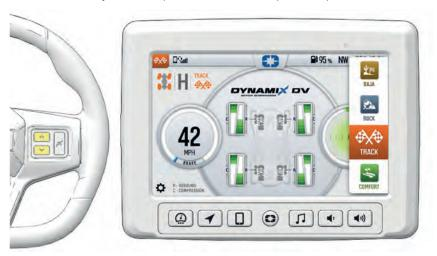
Notice the Mode Slide Out panel shows the active mode and the order/position. Ride Modes are described in more detail in the following sections.
