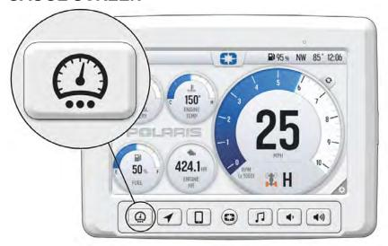
Press the Gauge Screen button to toggle between gauge screens. The display comes loaded with two different gauge screens. Additional gauge screens can be added or deleted.
