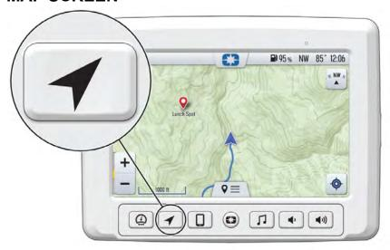
Press the *MAP SCREEN* button shown above to display the map screen. The map will center you based on the location of the GPS.
