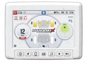
If your vehicle is equipped with Instantaneous Compression the suspension compression damping reverts to a firm base-damping setting with aggressive active vehicle events to respond to harsh terrain. If your vehicle is not equipped with Instantaneous Compression, all 4 shocks are set to the most firm setting.
