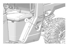
Always ensure that the fuel tank filler cap is fully tightened and secure before operating or transporting the vehicle.
