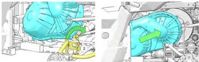
8. Install and torque the outer clutch cover bolts to specification.
