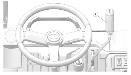
To change gears, stop the vehicle, and with the engine idling, move the lever ④ to the desired gear. Do not attempt to shift gears with engine speed above idle or while the vehicle is moving.
