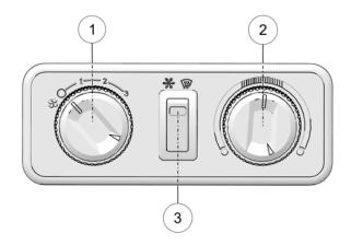
To operate the cab heater, rotate the fan control (1) to the desired fan speed setting. The far left setting turns the fan off.
