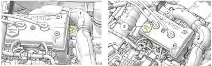
The oil dipstick is located on the engine. Access the dipstick through the right rear wheel well.
