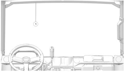
The safety labels ① are located on the front ROPS, above the driver's head.
