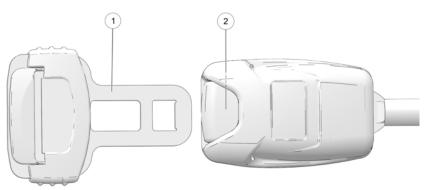
This vehicle is equipped with three-point lap and diagonal seat belts for the operator and any passengers. Always make sure the seat belts are secured for all riders before operating. The driver's seat belt is equipped with a seat belt interlock. Vehicle speed will be limited to 15 MPH (24 km/h) if the seat belt is not secured.
