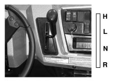
To change gears, stop the vehicle, and with the engine idling, move the lever to the desired gear. Do not attempt to shift gears with engine speed above idle or while the vehicle is moving.
