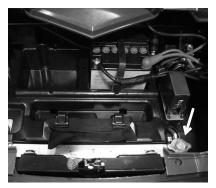
**NOTE:** Use of a non-standard pressure cap will not allow the recovery system to function properly. See your dealer for the correct replacement part.
