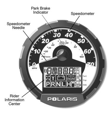
**NOTE:** In addition to showing vehicle speed, the speedometer needle flashes when a low fuel condition exists.
