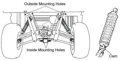
Rear Suspension Shown Adjustment is similar for Front Suspension
