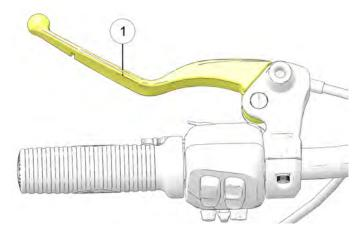
Freeplay (gap) is the amount of lever movement from the rest position to the point of cable resistance. Clutch lever freeplay should be 0.5-1.5 mm. Measure the gap between the clutch lever and the lever housing ②. Adjust clutch lever freeplay if necessary.
