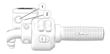
3. The fluid level should be above the minimum indicator mark ② near the sight glass.
