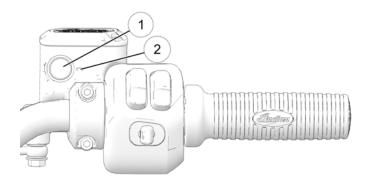
Reinstall the diaphragm, diaphragm plate, cover, and screws. If diaphragm is extended, return it to its collapsed or flattened position.
