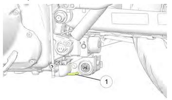
3. On models equipped with a passenger seat, remove the rear seat bracket bolt ②, washer, and nylon grommet.
