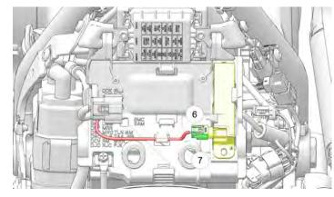
13. Install the Wireless Control Module (WCM) (§) onto the upper battery tray. Connect the main harness (§) to the WCM.
