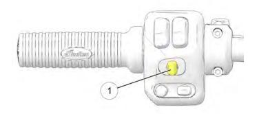
To activate the hazard switch, press on the center of the turn signal switch (1).
