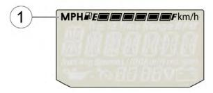
The segments of the fuel gauge ① show the level of fuel in the fuel tank. When the last segment clears, a low fuel warning is activated. All segments including the fuel icon will flash. Refuel promptly.
