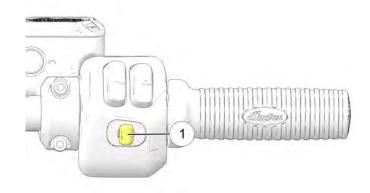
Cruise control can be activated and adjusted from the right control using the Cruise Control Switch ①.
