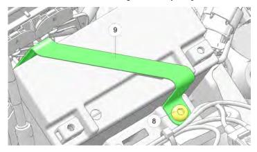
10. Remove the battery strap by moving the front of the strap forward out of the retention feature of the battery box.
