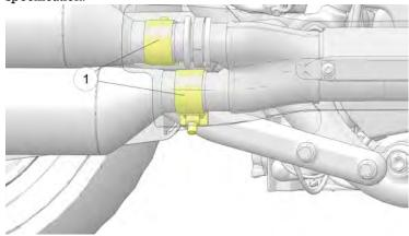
TORQUE 40 ft-lbs (54 N·m) Check the two muffler fasteners 1 on the exhaust support. Torque each fastener to specification.
