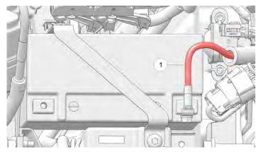
7. Insert the battery hold down strap into the battery box retention slot and slide the strap towards the rear of the bike.
