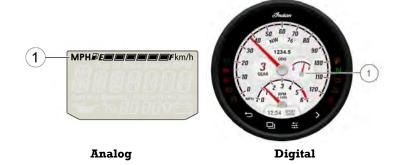
The segments of the fuel gauge ① show the level of fuel in the fuel tank. When the last segment clears, a low fuel warning is activated. All segments including the fuel icon will flash. Refuel promptly.
