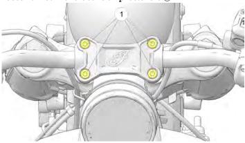
Rotate the handlebar into the desired position and torque the riser clamp fasteners to specification. The clocking dimples on both side of the handlebars should line up with the split in the risers.
