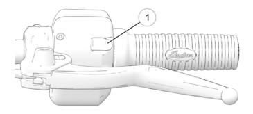
The power switch must be ON for the toggle switches to function. Use the right-hand switch to navigate through menus or accept dialog boxes on the Ride Command display. Use the left-hand switch to back out of menus, decline dialog boxes, hang up phone calls, and toggle through display screens.
