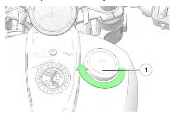
Turn the fuel cap counter-clockwise to remove it. If the fuel cap is equipped with a tether, carefully rest fuel cap on the tank so that the rubber bumper is contacting the tank. See page 88 for fueling instructions. To tighten the cap, turn it clockwise (shown above) until the seal compresses onto the tank, then continue to tighten until the cap ratchets several times.
