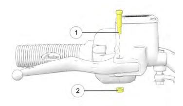
2. Install the pivot pin ①. Torque the pivot pin to specifications.
