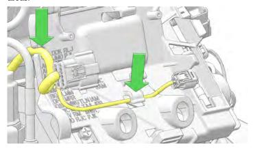
12. Install the antenna  $\mbox{\Large (6)}$  onto the upper battery tray. Connect the antenna harness  $\mbox{\Large (7)}$  to the antenna.
