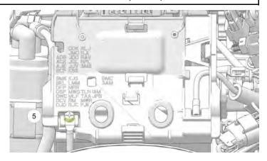
Install the antenna wiring harness onto the upper battery tray.
