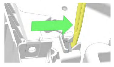
8. Install the battery hold down strap fastener  $\ \mathfrak{D}$  through the battery hold down strap  $\ \mathfrak{D}$ .
