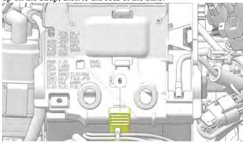
7. Lift the rear of the upper battery tray upward and pull it toward the rear of the unit to remove.
