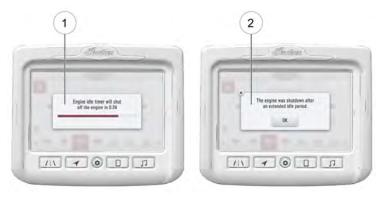
For motorcycles equipped with Ride Command, a notification will display a countdown timer to warn that the engine is about to shut off 1. After the time has elapsed and the engine is shut off, a subsequent notification will be displayed 2. After the engine shuts off, the engine can re-started by pressing the starter switch.
