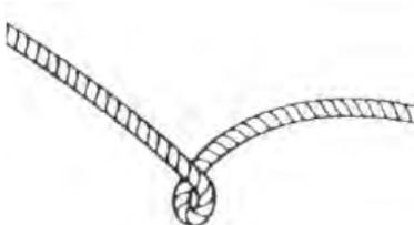
A kinked winch cable made of wire rope that has been “straightened out” is shown at right. Even though it may look usable, the cable has been permanently and severely damaged. It can no longer transmit the load that it could prior to kinking. Promptly discontinue use of a winch cable in this condition.
