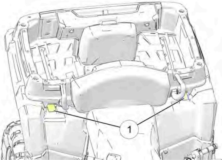
2. Lift the rear of the driver seat and slide the seat towards the back of the vehicle to remove it.
