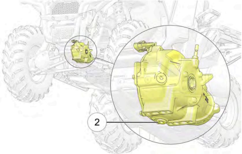
3. Put a drain pan below the drain plug.
