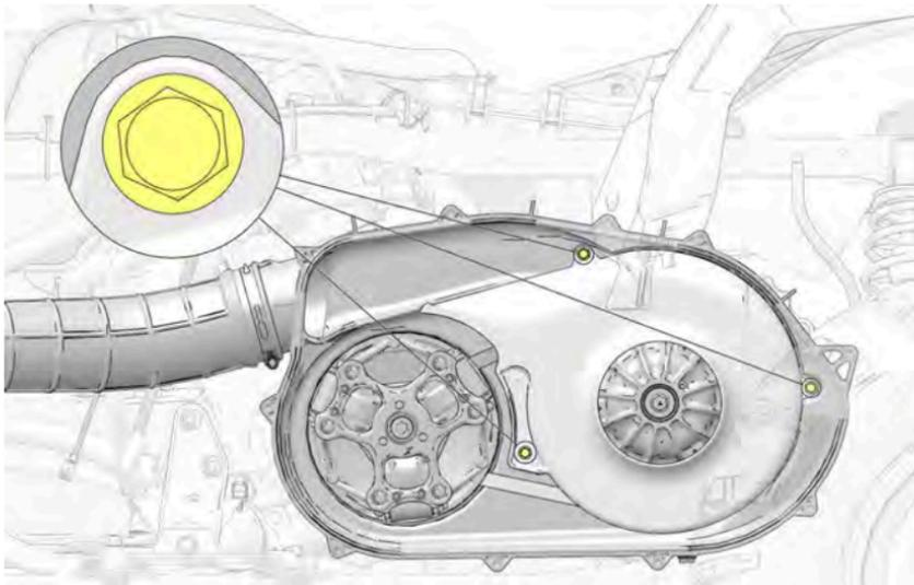
19. Install the outer PVT cover and 10 fasteners. Torque fasteners to specification.
