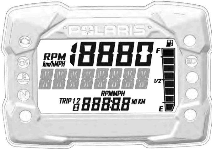
To toggle through available features, press Reverse Override / Mode Button ① from the left hand controls. For the full list of available features, see the Display Area 2 section of this chapter.
