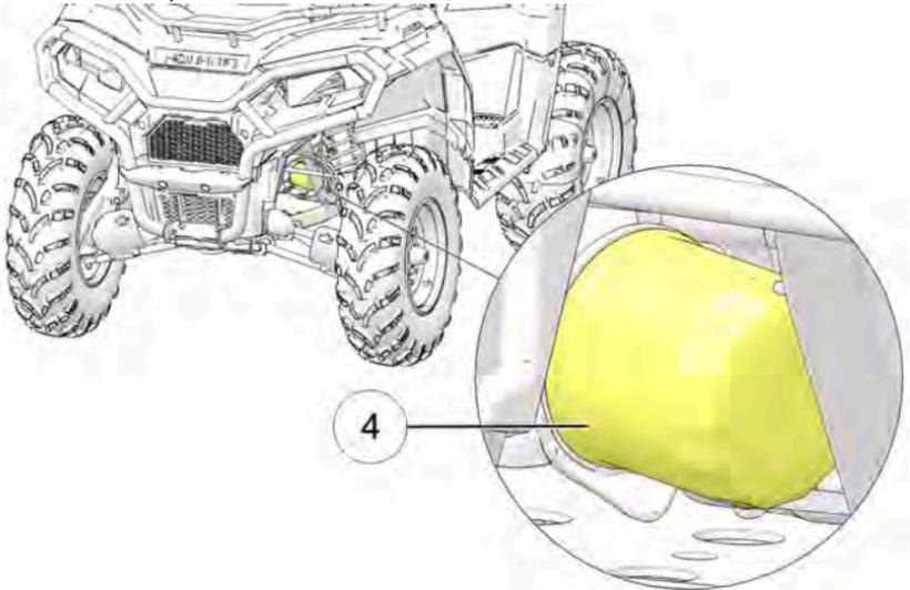
10. Remove the right side panels to gain access the oil filter. See page 170.
