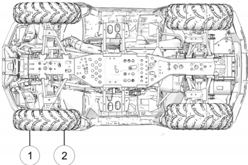
Use the following procedure to check the toe alignment of the vehicle. The recommended toe alignment is 1/4-1/2 inch (6-12 mm).
