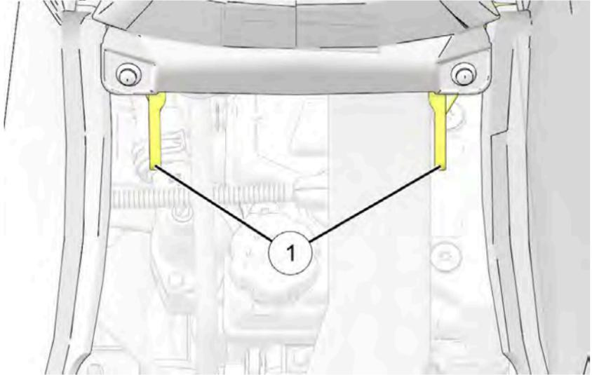
2. Slide the driver seat forward and lower the rear.
