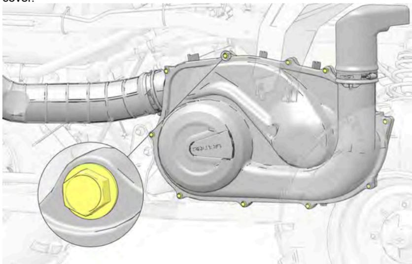
6. Using care, pull the outer PVT cover out the side of the vehicle.
