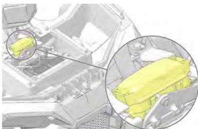
1. Open the front box cover, and remove the access panel.
