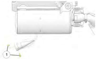
2. Remove the spark arrester ② from the end of the muffler.
