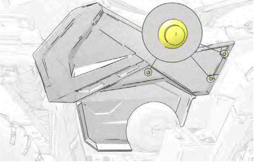
3. Grasp the rear of the side panel. With a firm motion, pull the side panel outward to disengage it from the vehicle.
