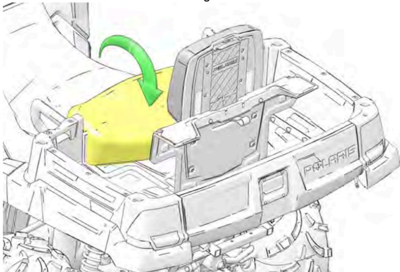
7. Test the passenger seat lockout by attempting to release the cargo box dump latch. If the dump latch releases, the seat is not secure. Repeat the set-up procedure. If the lock-out is not working properly, do not allow a passenger to ride the vehicle. See your POLARIS dealer for service.
