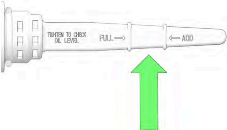
7. If needed, use a funnel to slowly add the recommended oil as indicated by the level on the dipstick. Do NOT overfill.
