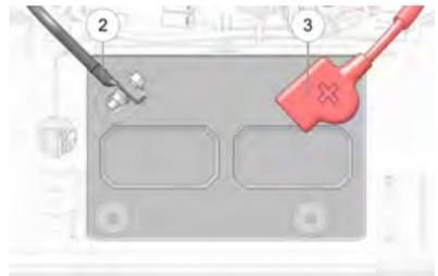
3. Disconnect the negative (-) black cable **②** first. Then disconnect the positive (+) red cable **③**.
