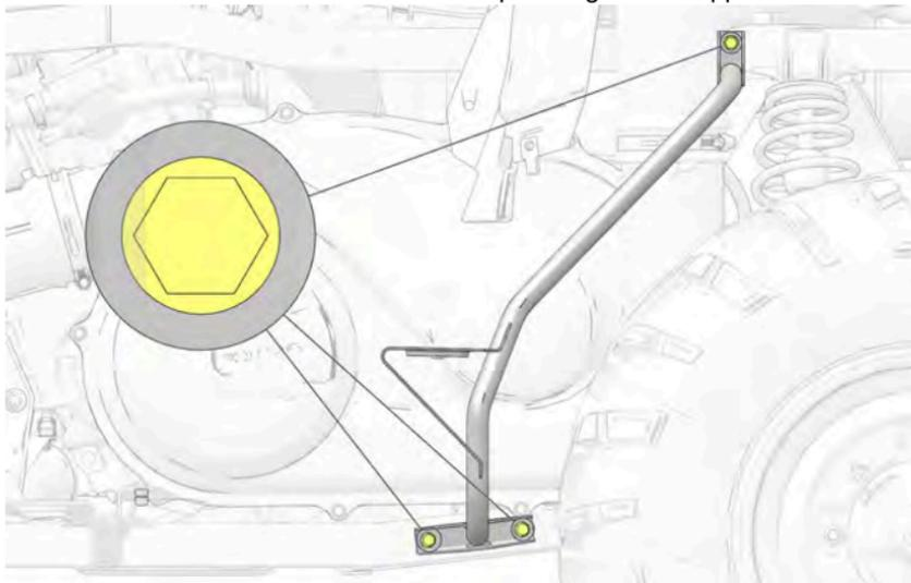
5. Remove the 10 fasteners securing the outer PVT cover to the inner PVT cover.
