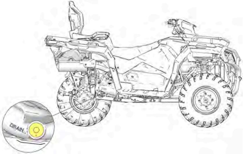
7. Clean any dirt or debris on the drain plug. Inspect the o-ring and replace if necessary.
