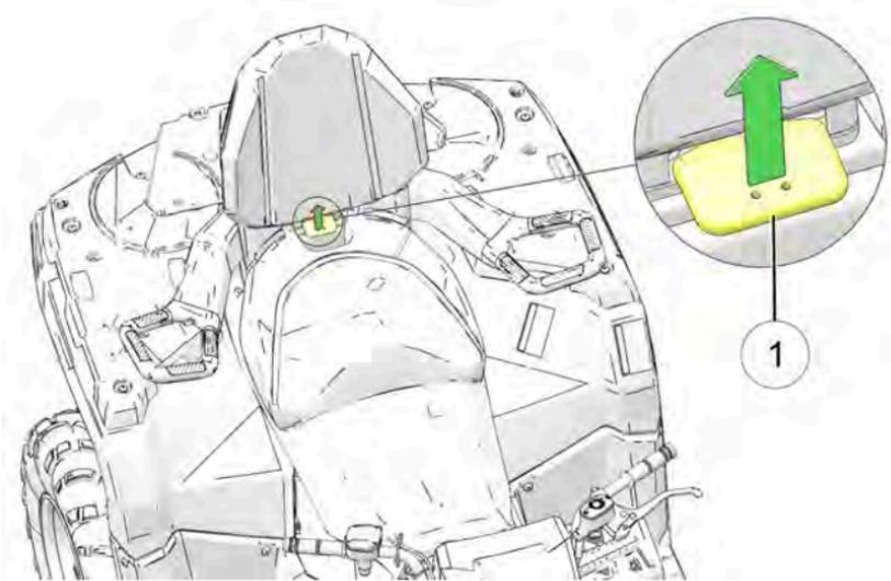
2. Tilt the passenger seat forward and then lift up to remove the seat from the vehicle.
