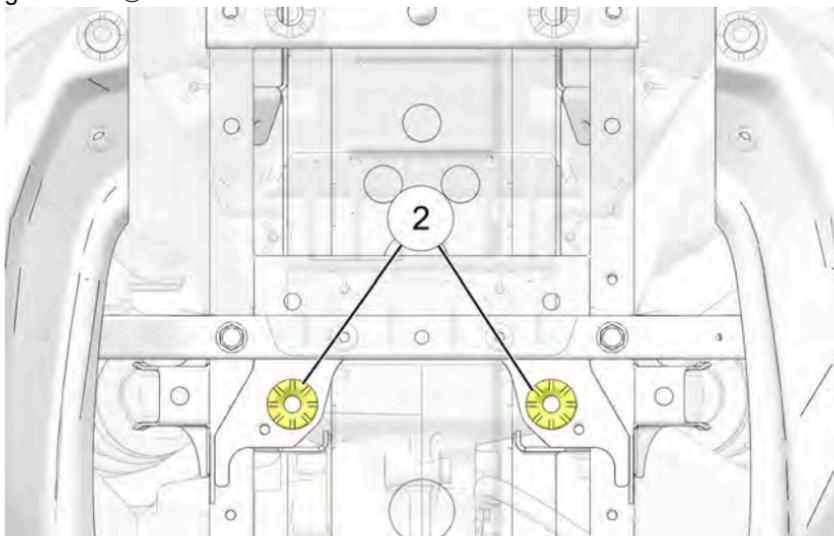
4. Install the passenger seat onto the vehicle by pushing back on the backrest and down on the passenger seat latch lever ③ until you feel and hear a click.
