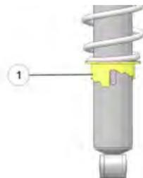
Vehicle loads affect suspension spring pre-load requirements. Use the Shock Spanner Wrench included in the vehicle's tool kit to adjust pre-load as necessary to avoid bottoming of the shocks.
