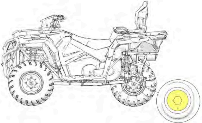
4. If needed, use a funnel to slowly add the recommended fluid to bring the level to the bottom of the fill hole threads.
