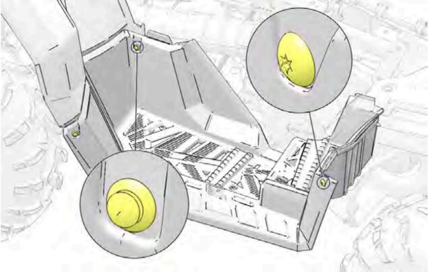
6. Remove the six screws and nuts from the bottom of the footwell. Pull the footwell downward and outward to remove it.
