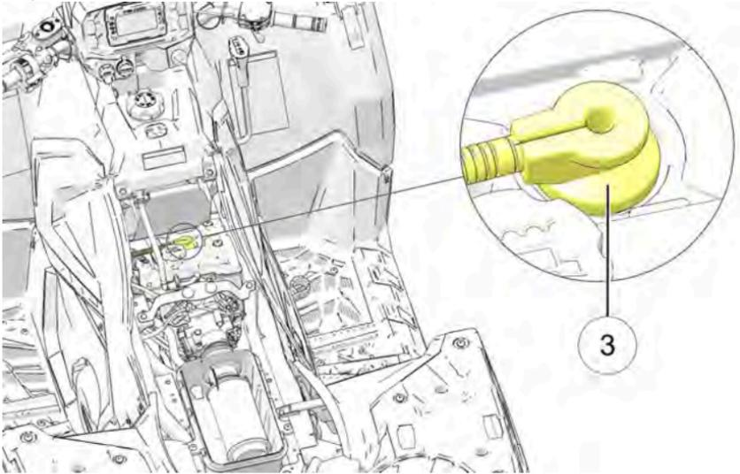
6. Remove the spark plug cap from the spark plug by rotating the cap 1/4 turn and pulling it upwards.
