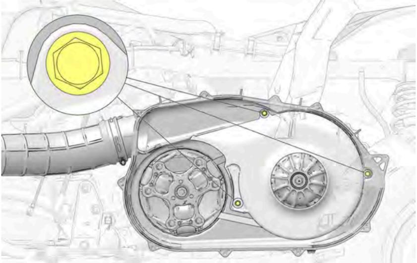
8. Note the orientation of the drive belt so that it can be installed in the same direction.
