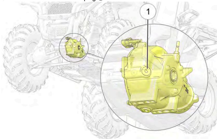
3. Remove the fill plug and check the fluid level. The fluid level is correct if fluid is visible at the fill hole threads.
