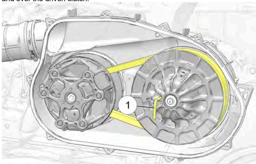
15. Rotate the driven clutch and walk the belt into the clutch.
