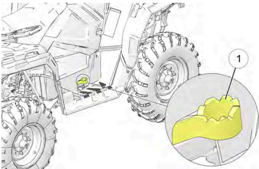
The auxiliary brake system is intended to be used as a backup for the main brake system. Should the main system fail, use the auxiliary foot brake ①.
