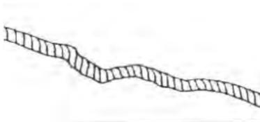
A winch cable made of synthetic rope should be inspected for signs of fraying. Replace the cable if fraying is observed (shown below). Promptly discontinue use of a winch cable in this condition. Also replace the winch cable if there are frayed or melted fibers. Such an area of the synthetic rope will be stiff and appear smooth or glazed. Promptly discontinue use of a winch cable in this condition.
