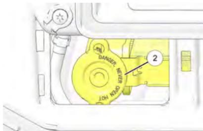
4. Use a funnel to slowly add the proper amount of recommended coolant through the radiator filler neck.
