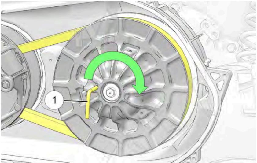
10. Carefully walk the belt off the driven clutch and remove from the drive clutch.
