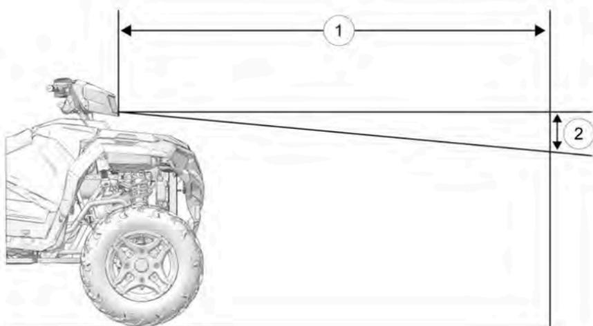
1. Position the vehicle on a level surface with the headlight approximately 25 ft (7.6 m) from a wall ①. Place the transmission in PARK.
