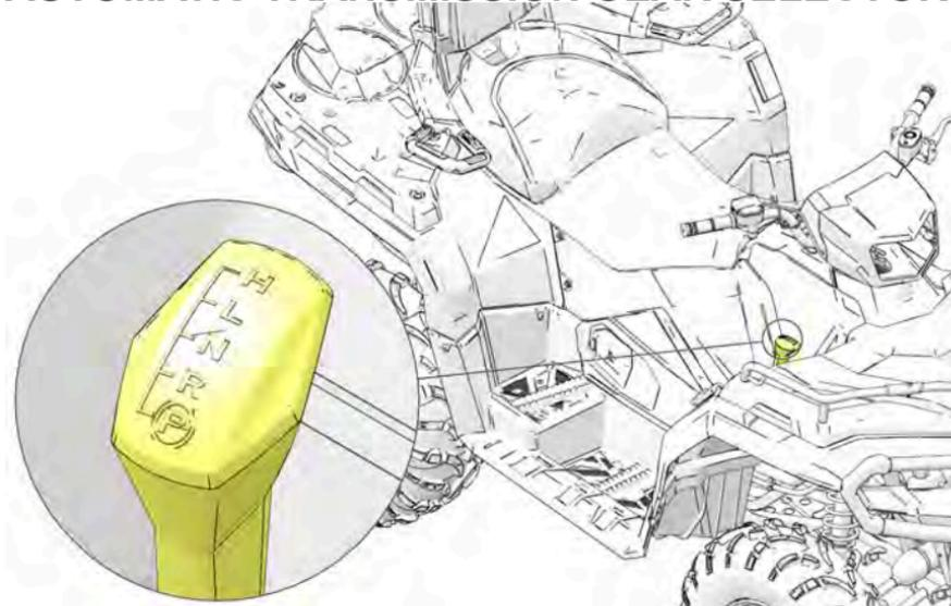
The transmission gear selector is located on the right side of the vehicle.
