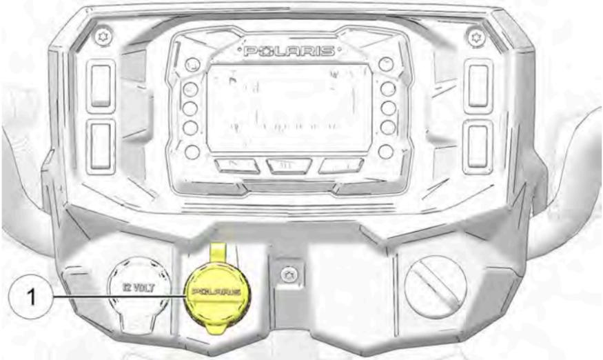
Polaris recommends maintaining battery charge by using a Polaris battery trickle charger or by charging once a month using the battery charge port ①. The Polaris offered battery trickle charger can be left connected during the storage period, and will automatically charge the battery if the voltage drops below a pre-determined point. See the Polaris Products chapter for the part number.
