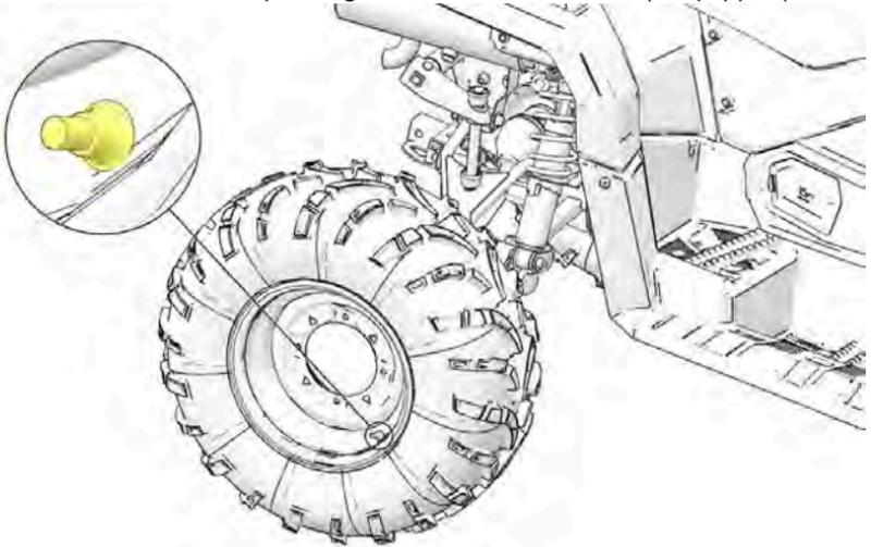
3. Install the wheel nuts ① and finger-tighten them.
