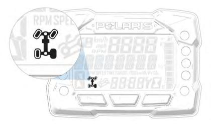
The All Wheel Drive (AWD) system is controlled by the Driveline switch. Engage AWD before getting into conditions where front wheel drive may be needed. If the rear wheels are spinning, release the throttle before switching to AWD.
