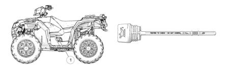
Check the oil level when the engine is cold. Never check the oil with the engine running.
