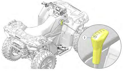
The transmission gear selector ② is located on the right side of the vehicle.
