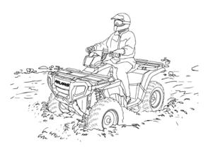
After leaving water, test the brakes. Apply them lightly several times while driving slowly. The friction will help dry out the pads.
