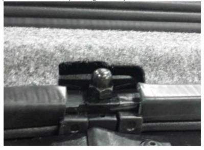
Attach the clamps on both sides of the window tor the door frame using two (2) rivets per clamp
