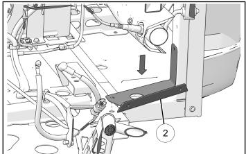
6. Attach right bottom mud guard to side mount using one screw (8). Torque screw to specification.
