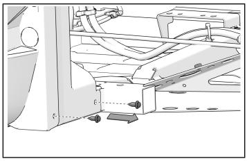
7. Align left mud guard ① with holes in fender and chassis bracket lower brace.
