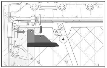
3. Attach right cargo mud guard to cargo box using two screws ⑦. Torque screws to specification.
