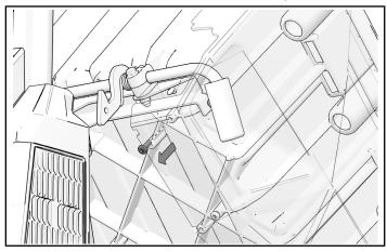
3. Align left cargo mud guard ③ with holes on cargo box mounting surface as shown.
