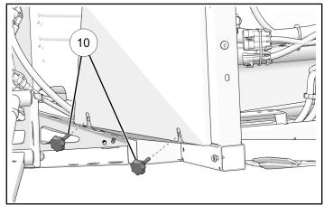
10. Install cap 6 into end of chassis tube.
