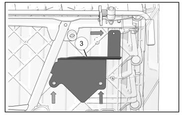
4. Attach left cargo mud guard to cargo box using three screws ⑦ and two washers ⑧. Torque screws to specification.
