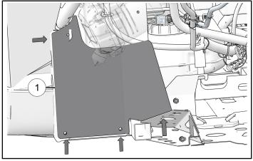
8. Attach left mud guard using two knobs (10) and two push-pin rivets (14). Hand tighten knobs.
