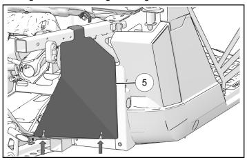
9. Attach right side mud guard using two knobs 10. Hand tighten.
