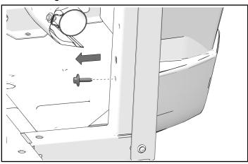
5. Align right bottom mud guard ② with holes in chassis.
