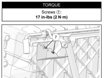
4. Remove and discard screw from chassis side mounting surface.
