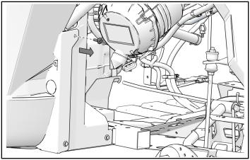
6. Remove and discard two push-pin rivets.
