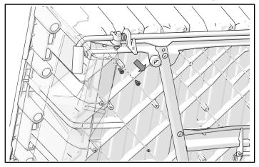
2. Align right cargo mud guard ④ with holes on cargo box mounting surface as shown.
