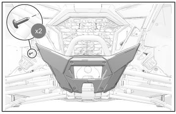
2. Reinstall bottom front fascia with retained fasteners (shorter).
