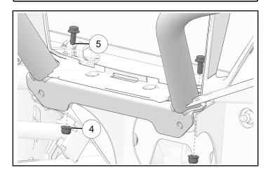
2. Install front of bumper with two bolts (5) and two nuts (4). Counter-hold nuts and torque two bolts to specification.
