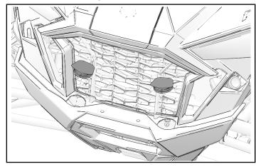
2. Remove two top mounting fasteners (longer) and two bottom mounting fasteners (shorter) to remove front fascia from vehicle.
