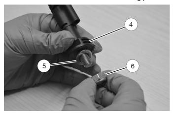
6. Install mounting pins 4 and washers through holes on mounting base 2.
