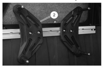
8. Tighten four screws (1) to specification.
