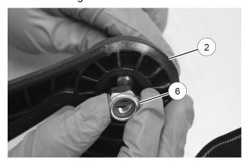
8. Tighten mounting pins ④. Tighten until mounting pin is tight and flats on mounting pin line up with lines on mounting base ②.
