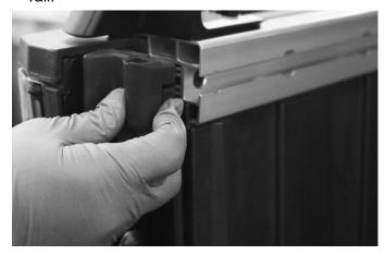
5. Install mounts ② to rail. T-nuts ④ will slide into opening in rail.
