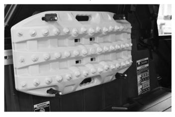
7. Carefully remove traction boards from mounts ②. Make sure not to move mounts along rail.
