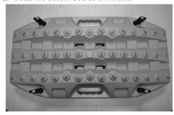
3. Turn tabs on each mounting pin 4 to lock traction boards on mounts.
