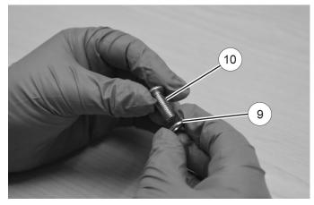
2. Assemble two flat washers (8) to two screws (10).
