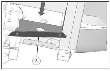
5. Loosely install right bottom mud guard to side mount using one screw ③.
