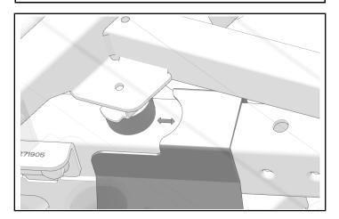
9. Attach using two knobs 4. Hand tighten.
