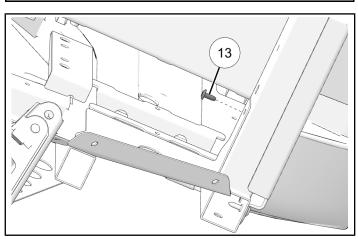
6. Loosely install right bottom mud guard to chassis tube using one screw ① and one nut ⑤
