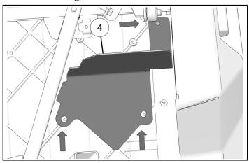
4. Attach left cargo mud guard using three screws ② and two washers ⑥. Torque screws to specification.
