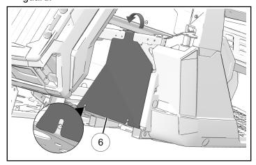
9. Attach right side mud guard using two knobs (4). Hand tighten.
