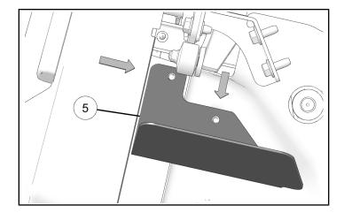
3. Attach right cargo mud guard to cargo box using two screws ①. Torque screws to specification.
