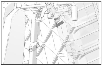
3. Align left cargo mud guard ④ with holes on cargo box mounting surface as shown.
