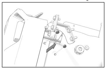
2. Align right cargo mud guard ⑤ with holes on cargo box surface as shown.
