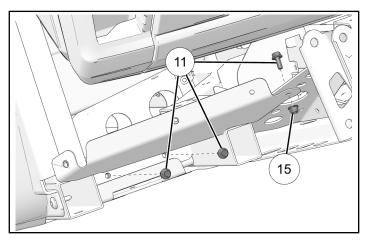
8. Install left side mud guard ①. Make sure top of mud guard is fitted to chassis tube. Make sure to align with holes in left bottom mud guard.
