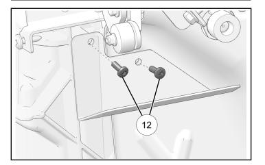
4. Put right bottom mud guard 3 onto chassis.
