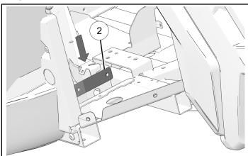
7. Attach left bottom mud guard to chassis and bottom nut plate using three screws ① and one nut ⑤. Torque screws and nut to specification.
