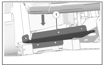
6. Put bottom nut plate ② behind left bottom mud guard and chassis bracket lower brace.
