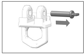
2. Install retaining bolt through shackle ② and shackle mount on bumper. Tighten retaining bolt.
