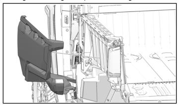
2. Install kept upper cargo box push pin rivet.
