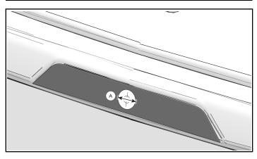
4. Use a cutting tool to make a notch at the top of the drilled hole where marked.
