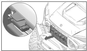
2. Put template ② on center of front facsia. Use a cutting tool to mark the center so it is visible when the template is removed.
