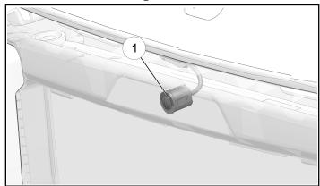
6. Push camera ① until two locking clips are fully seated.
