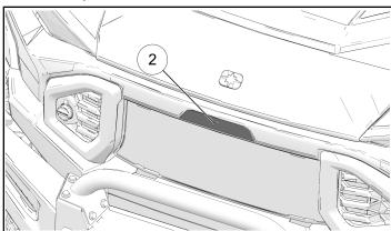
3. Remove template and drill a hole through front fascia where center was marked.
