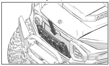
2. Push top of grille in until two tabs engage front fascia and it is fully seated.
