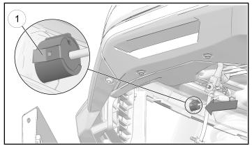
7. Connect camera connector to Ride Command® audio harness connector.
