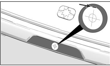
5. Install front camera ① into hole.
