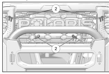
3. Torque screws ② to specification.
