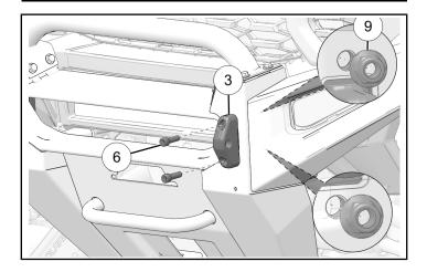
2. Torque nuts 9 to specification.
