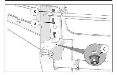
5. Torque bracket hardware to specification.
