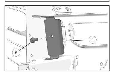
4. Loosely install bracket to bumper using two screws6 and two nuts 8.
