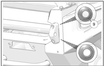
3. Loosely install bracket ① to rear of shackle mount using one screw ⑥.
