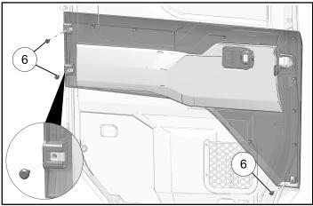
7. Torque screws 6 to specification.
