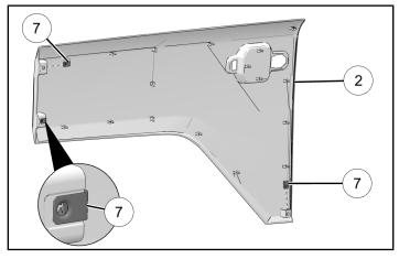
4. Install interior accent panel ④ onto interior of front left door (Kit P/N 2889075). Align plastic clips with slots in door. Push panel firmly into place.
