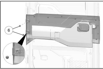
7. Torque screws 6 to specification.
