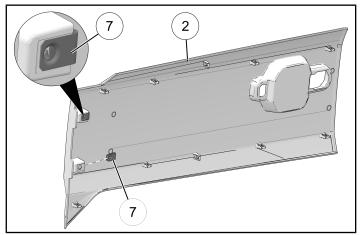
Install interior accent panel ④ onto rear left door (Kit P/N 2889076). Align plastic clips with slots in door. Push panel firmly into place.
