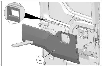
Install exterior accent panel 2 onto exterior of front left door. Align plastic clips with slots in door. Push panel firmly into place.
