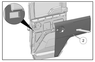
6. Attach exterior accent panel ④ using three screws⑥.
