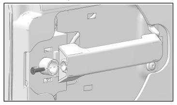
3. Remove and keep door handle. Pull handle out from hinged pivot.
