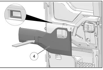
5. Install exterior accent panel ② onto exterior of rear left door. Align plastic clips with slots in door. Push panel firmly into place.
