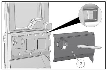
6. Attach exterior accent panel ④ using two screws⑥.
