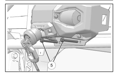
4. Torque four nuts 6 to specification.
