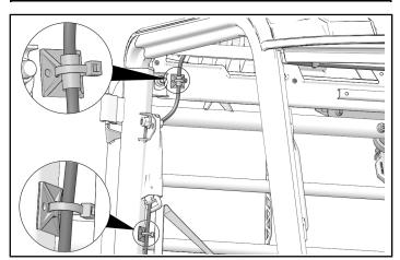
4. Attach wiring to vehicle frame using adhesive clip and edge clips. Hold clips firmly in place for 30-seconds.
