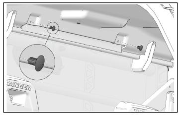
2. Remove and keep four screws at rear of roof.
