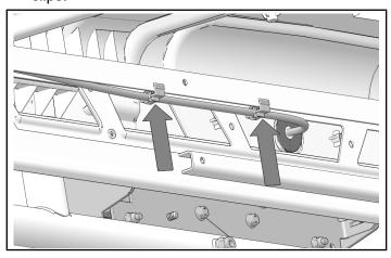
2. Attach wiring at corner of vehicle roof brace using push dart clip.
