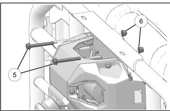
2. Route wiring harness through hole in roof until grommet ② can be installed in hole.
