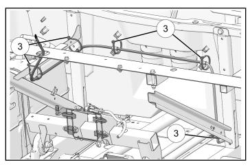
7. Route harness under vehicle floor. Attach to main wiring harness using cable ties ③.
