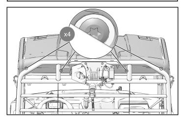
13. Put roof liner in place. Install two push dart clips ④ in roof liner.
