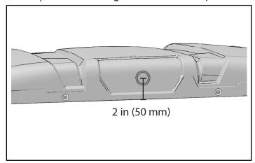
4. Lift roof up away from vehicle. Drill a hole at marked point. Replace roof.
