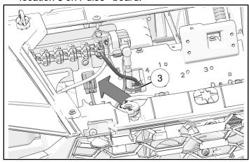
10. Connect wiring to Pulse® bar.
