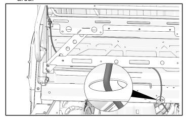
6. Route harness along front edge of seat mount area. Attach to underside of seat mount structure using cable ties ③.
