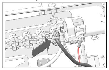
11. Connect positive and negative ring terminals to Pulse® bar. Torque nuts to specification.
