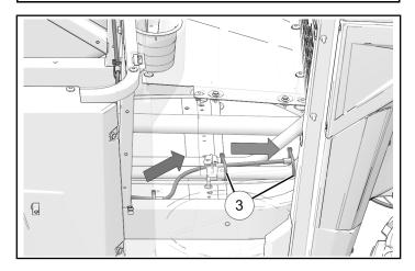
8. Route harness up to underhood area along existing battery cables. Attach using cable tie ③. Make sure wires are kept away from moving parts.
