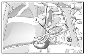
9. Route through opening in Pulse® board. Attach to frame using cable tie ③. Attach fuse holder to location **6** on Pulse® board.
