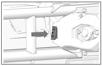
Push the top button of the switch "IN" to spool line in to winch. Push the bottom button of the switch "OUT" to spool line out from winch.
