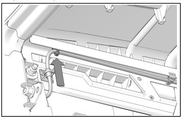
3. Attach wiring to vehicle frame behind passenger door opening using adhesive clips. Hold clips firmly in place for 30-seconds.
