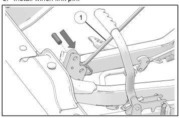
7. Install cotter pin into winch link pin.
