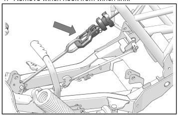
2. Remove and keep cotter pin from winch link pin.
