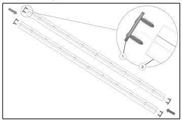
2. Align screw holes on rail with holes in rack in desired location. Attach using six screws ③.
