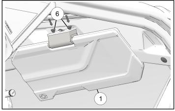
8. Check fitment of visor panels by opening and closing along hinge. Adjust pressure screw (A) as necessary.
