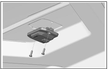
7. Attach left visor panel assembly ① to visor mounting brackets using two screws ⑥. Torque screws to specification.
