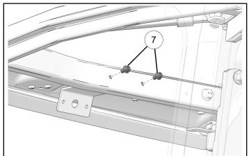
4. Put visor mounting brackets through trimmed openings in roof liner.
