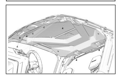
6. Install kept screws into middle of roof liner. If equipped, install dome light using two retained screws and connect any wiring.
