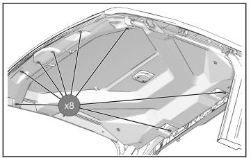
2. Remove two screws from middle of roof liner. If equipped, remove dome light and disconnect any wiring.
