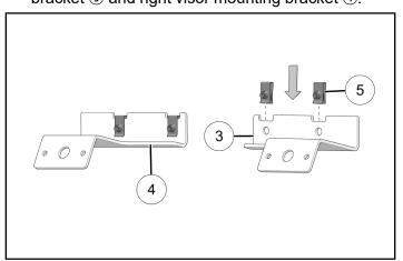
3. Install visor mounting brackets on ROPS front visor bracket using two screws ①. Torque screws to specification.
