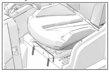
Push down on back of seat to latch seat into frame. Lift up on seat to make sure it is fully installed.
