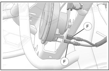
17. Attach cables tie on horn harness to vehicle harness.
