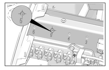
2. Connect harness ② fuse holder **2F** with push-dart clip into location **5**.
