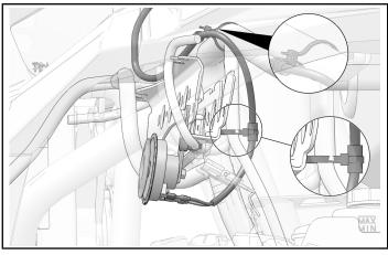
18. Attach two cable ties ④ onto horn harness. Use cable ties to attach to vehicle harness.
