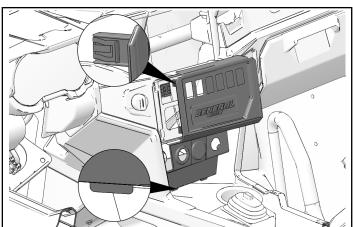
9. Route connector **8F** through center console opening. Connect to horn switch ③.
