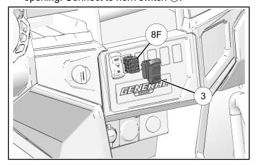
10. Install connected switch into center console ③ until fully seated.
