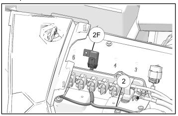
3. Remove cap from any slot on Polaris Pulse® Bar. Connect connector **3F** to open slot.
