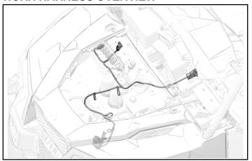
Drill hole onto location 5 behind Polaris Pulse® Bar.
