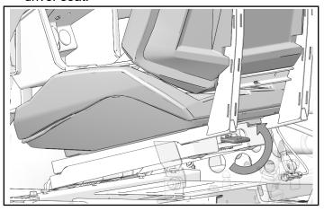
2. Lift up and forward on seat while lifting up on latch lever to remove from vehicle.
