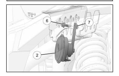
14. Install clip edge ⑤ onto horn. Route vehicle harness into clip edge.
