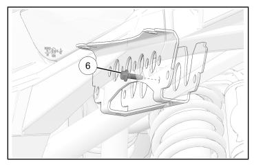
13. Install horn ② loosely with one screw ⑥ and one washer ⑦ onto cross member.
