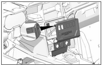
7. Cut out one opening on center console. Make sure to cut out to the outer most rectangle line.
