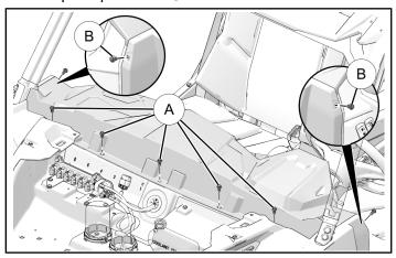
3. Move panel upward and rearward, detaching eight spring clips ©.
