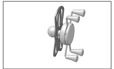
4. Install x grip onto mount arm. Tighten mount arm knob.
