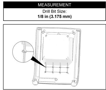
2. Turn over panel. Install phone mount ① onto the panel with eight screws ② and eight washers ③. Hand tighten screws until fully seated.
