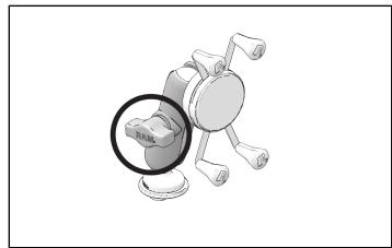
2. Install phone mount assembly onto phone mount through the middle hole. Move phone mount assembly to location as desired.
