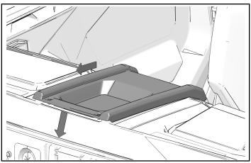
2. Install two push-pin rivets.
