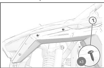
3. Remove and keep three hood fasteners.
