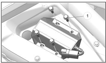
3. Secure four screws ① with four nuts ②. Torque to specification.
