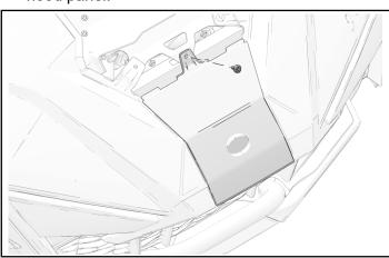
2. Remove and keep three front fender fasteners.
