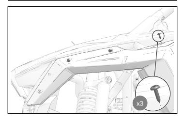
3. Install front hood panel with one retained fastener.
