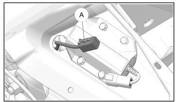
5. Connect main wire harness connector (A) to RIDE COMMAND+ Plug-In connector.
