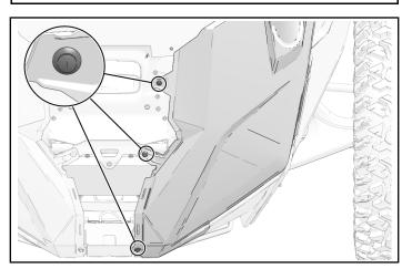
2. Install three retained front fender fasteners. Torque hood and fender fasteners to specification.
