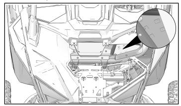
Install RIDE COMMAND+ Plug-In and four screws
