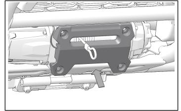
10. Install four screws. Torque screws to specification.
