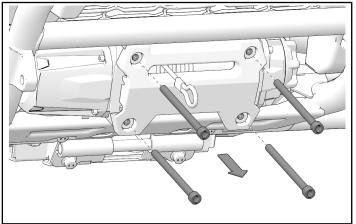
3. Remove and keep four screws that attach fairlead to winch.
