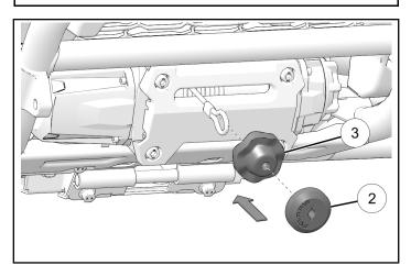
13. Install hook on winch rope with clevis and cotter pin.
