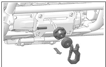
2. Remove and keep four screws that attach winch to vehicle. Winch will remain in vehicle.
