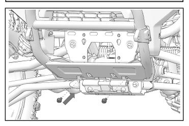
4. After all screws are installed, torque all fasteners to specification.
