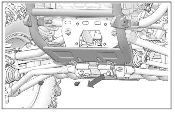
2. Remove four screws and nuts from the upper mounting points.
