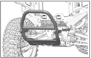
2. Install four screws and four nuts at upper mounting points.
