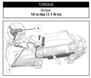
7. Locate white connector on existing winch harness. Remove cap from connector and connect sensor bar to harness.
