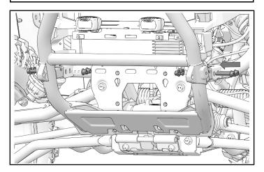
3. Install two lower screws in bull bumper.
