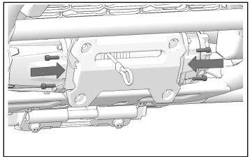
11. Install four winch mounting screws. Torque screws to specification.
