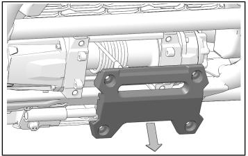
5. Remove and keep one screw from top of winch.
