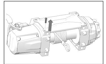
6. Route wiring for sensor bar ① through clip ④. Attach clip to winch with screw removed in previous step. Clip must face downward. Torque screw to specification.
