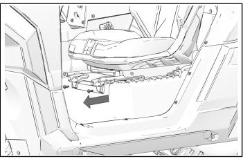
2. Lift front of seat and pull forward to remove seat.
