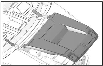
2. Pull the rubber straps down over the hooks to secure the hood.
