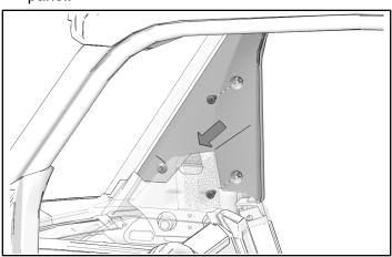
4. Pull outer sail panel outward, and rotate inner and outer sail panels toward the front of the vehicle. Remove outer sail panel only.
