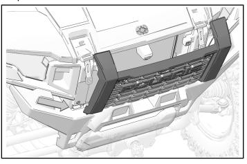
4. Push each stud in and turn one-quarter turn clockwise to secure the grill.
