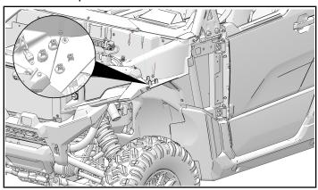
2. Install RIDE COMMAND+ Plug-In with four screws ①. Torque to specification.
