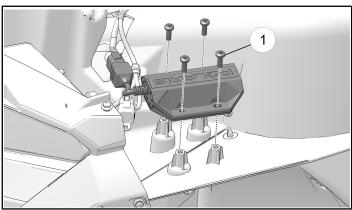
3. Connect RIDE COMMAND+ Plug-In to chassis harness 6F.
