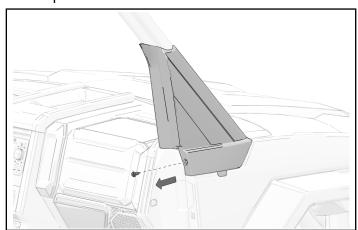
3. Remove and keep two screws from the inner panel.
