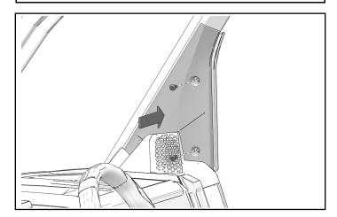
3. Install push-pin rivet.
