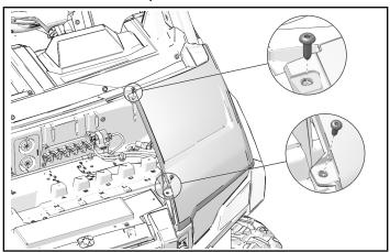
5. Pull fender outward to disengage upper tabs.
