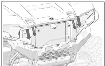
3. Insert tabs on the grill through the openings in the front fascia. Push the top of the grill into the proper position.
