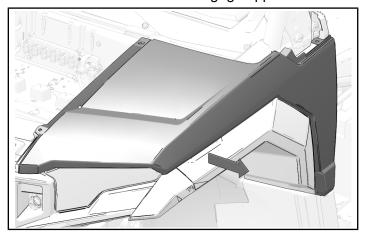
6. Rotate fender and lift to disengage lower tab and remove fender.
