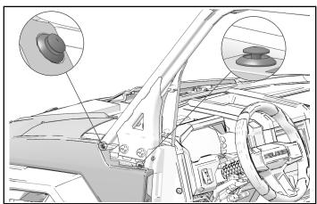
3. Remove and keep two push pin rivets from top of front fender.
