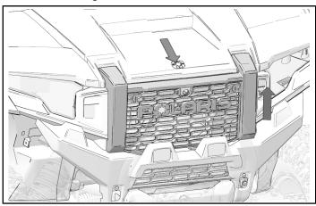
3. Unhook the rubber straps for the hood. Lift the hood to remove.
