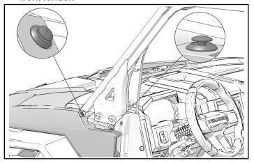
4. Remove and keep two screws from front fender.
