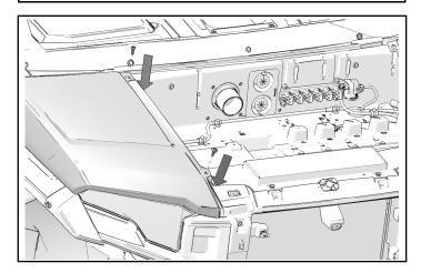
4. Install four push pin rivets.
