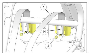
2. Install rear outboard harness clip to vehicle mount bracket using bolt ③ and nut ④ as shown. Make sure harness clip is on OUTBOARD side of mount bracket. Torque to specification.
