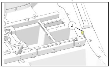
4. Install both front harness clips to seat mounting frame using one retained screw ① and two new screws ⑤ as shown. Torque screws to specification.
