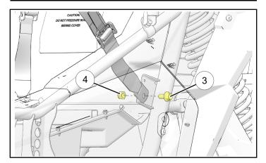
3. Remove and keep one screw ① from front outboard corner of seat mounting frame as shown.
