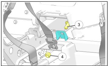
2. Install clip to vehicle mount bracket using bolt ③ and nut ④. Make sure harness clip is on FRONT side of mount bracket. Torque to specification.
