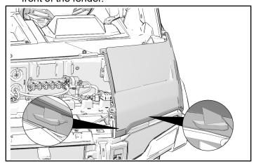
8. Install two retained left front fender screws. Torque screws to specification.
