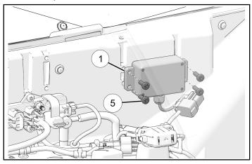
5. Install wireless remote holder ③ with two screws④.
