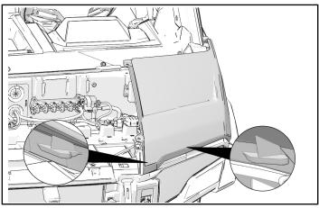
3. Remove two screws from the autostop receiver. Disconnect connector and remove autostop receiver.
