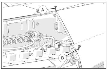
2. Pull up fender to disengage the two tabs in front of the fender.
