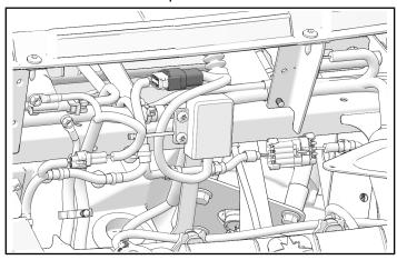
2. Remove two autostop receiver screws and autostop receiver.
