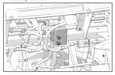
3. Install autostop receiver ① onto bracket with four screws ⑤. Torque until full seated
