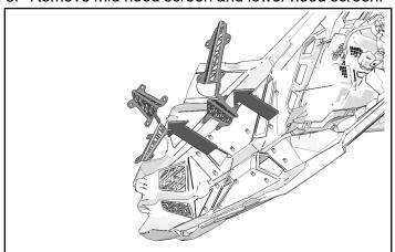
4. Install lower hood screen ① and mid hood screen② onto mounting studs.
