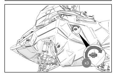
Twist hood fasteners counterclockwise to release hood.
