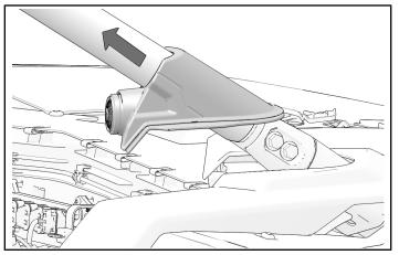
2. Feed fish tape (or equivalent) into opening of lower brace and up A-pillar, toward top cross-beam.
