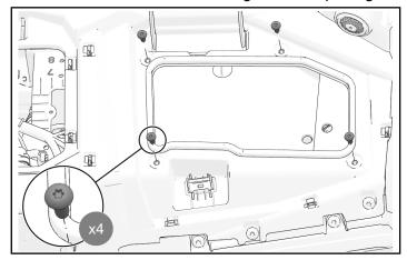
3. Remove and keep three front dashboard fasteners around glove box opening.
