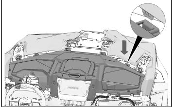
3. Make sure both rubber boots are properly seated around hood panels. Only upper lip should be visible, as shown with inset.
