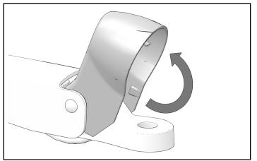
7. Place wiper arm onto wiper arm shaft in a position that will allow wiper blade to fully clean windshield.
