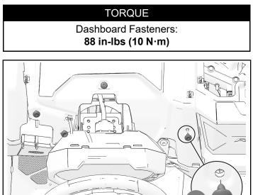
7. Open glove box lid and reinstall storage compartment. Install four retained dashboard fasteners around glove box opening.
