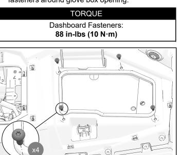
8. Install front of dashboard with three retained dashboard fasteners.
