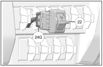
6. Push switch (2) into lower dash panel until tabs snap into place. Note switch orientation shown in graphic.
