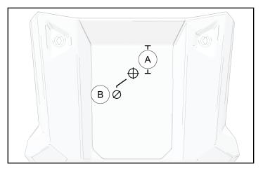
2. Remove nut from washer nozzle assembly. Pass nozzle (2) through hood panel and secure with nozzle nut.
