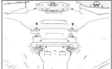
7. Carefully lift edge of left front hood panel to release tab from dashboard top as shown.
