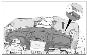
9. Carefully keep panels up-and-away from tabs and remove dashboard top by tilting rear section up and pulling out toward rear.
