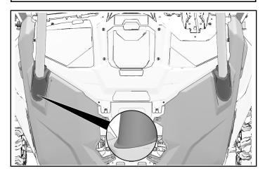
4. Reinstall two retained front dashboard fasteners into front edge of top dashboard.
