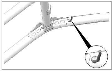
4. Tape ROPS harness (25) to fish tape and pull harness through holes and out opening in lower brace.
