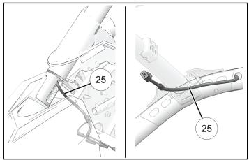
5. Secure ROPS harness to vehicle with edge clip 1.
