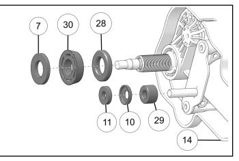
3. Pass wiper arm shaft and arm stopper shaft through windshield frame and attach with the following:
