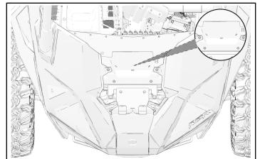
2. With a utility knife, carefully cut around edges of indentation.
