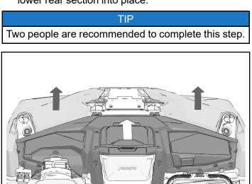
Make sure tabs on panels are aligned in slots on dashboard top. (Passenger-side panel shown; driver-side panel similar.)
