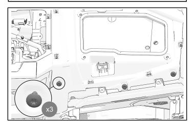
4. Tilt steering wheel down. Remove and keep four dashboard fasteners from dashboard surrounding steering wheel.
