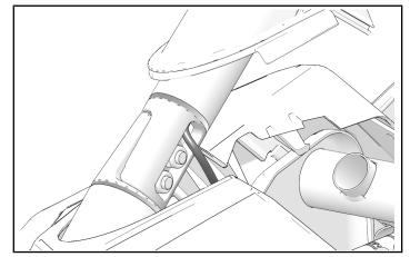
3. Locate fish tape and pull from round opening, as shown.
