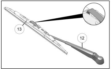
6. Lift wiper arm cap to reveal mounting bracket.
