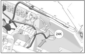
4. Remove switch blank from lower dash panel.
