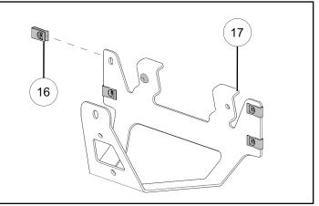
4. Install one U-clip nut 16 onto vehicle chassis.
