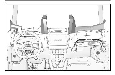
2. Open glove box lid. Remove and keep four dashboard fasteners around glove box opening.
