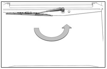
8. Attach wiper arm with washer ③ and nut ②.
