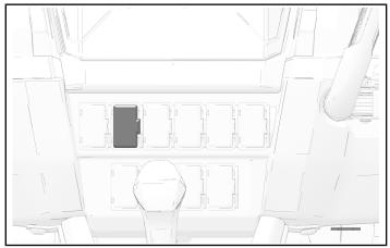
5. Route switch connector 24G below accessory mounting panel to switch opening and connect to switch @.
