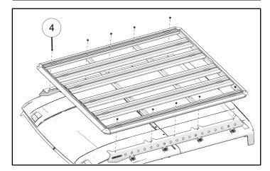
5. Use torque tool provided with platform rack kit to torque all top screws (4) until clicking sound.
