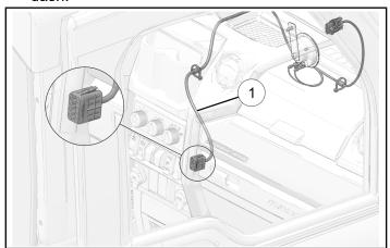
2. Route harness ① with spade and pulse connectors through grommet.
