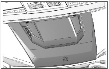
2. Rotate control panel trim rearward and down to remove top two tabs from vehicle.
