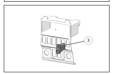
Connect switch connector on harness ① to switch
