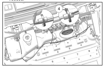
5. Attach horn harness ① to other installed harnesses with cable ties ④, as needed.
