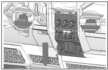
3. Remove center dash HVAC control panel trim and assembly. Disconnect any connections if needed.
