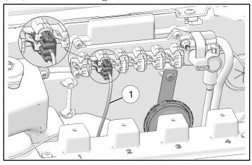
4. Attach horn harness ① using two cable ties ④ as needed.
