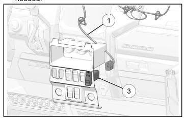
8. Install center dash onto vehicle with two push-pins rivet. Make sure horn switch ③ is fully seated.
