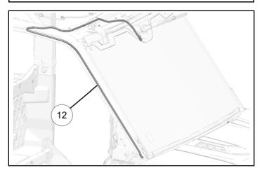
2. Pass washer fluid hose through slot on ROPS tube and install to front visor top bracket using four fir tree clips <sup>(8)</sup>.
