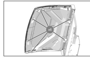
2. Remove and discard two screws. Remove roof liner.
