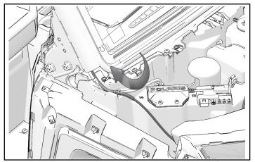
12. Pull harness through opening in ROPS above passenger opening. Route wiring as shown. Attach to roof using edge clips.
