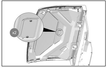
3. Locate trim line on inside of roof liner. Cut out hole along trim line.
