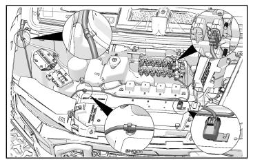
10. Connect **3F** to Pulse bar. Attach fuse **2F** in position shown
