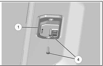
16. Install three fender screws.
