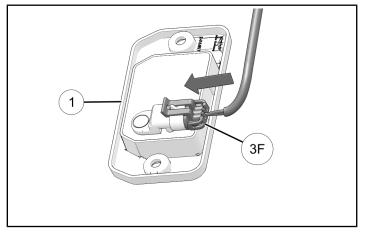
15. Install dome light ① to roof and attach using two screws ④. Tighten until fully seated.
