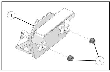
6. Install assembly onto the rail using Lock & Ride MAX® latching assembly.
