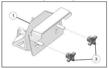
5. Install two nuts 4 until fully seated on to mount 1 studs.
