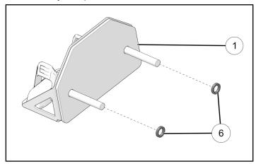
2. Install support mount ② onto mount ① studs.
