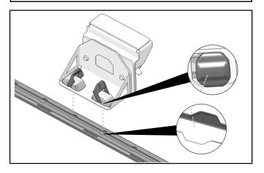
7. Attach assembly to rail by locking the Lock & Ride MAX® latching assembly.
