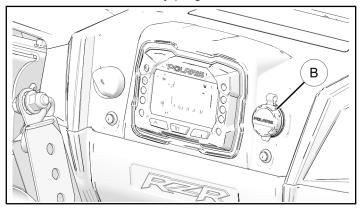
6. Disconnect wiring from 12V accessory plug.
