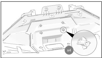
4. Put plug-in assembly in position on four mounting bosses. Make sure connector is pointed toward passenger side.
