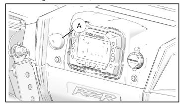
4. Lift up slightly on locking tab and disconnect wiring from ignition switch.
