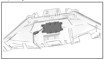
5. Attach plug-in assembly to dash using four screws②. Tighten until fully seated.
