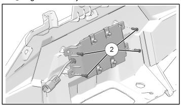
6. Locate plug-in connection under dash. Connect plug-in when installing dash.
