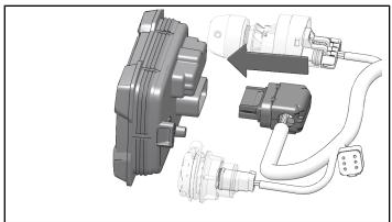
5. Connect wiring to 12V accessory plug.
