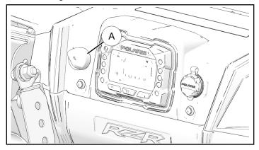
3. Connect wiring to ignition switch until it clips into place.
