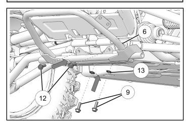
4. Loosely assemble left bracket ② and right bracket ④ to plow mount and bull bumper. Use four screws ⑫ and four nuts ⑪ to attach brackets to plow mount. Use two screws ⑩ and two nuts ⑦ to attach brackets to bull bumper.
