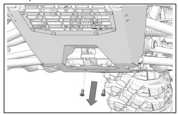
2. Remove two screws from front tow cover.
