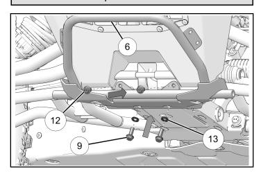
4. Loosely install two button head screws ® and two nuts ①.
