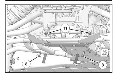
5. Loosely install left bracket ①, right bracket ③, eight nuts ⑪, and eight screws ⑫.
