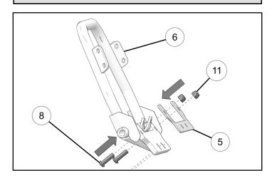
2. Remove two lower bolts from tow cover on vehicle.
