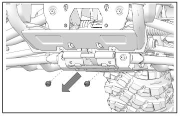
3. Loosely install mount **(6)**. Use two screws **(9)**, two washers **(3)**, and two screws **(2)**.
