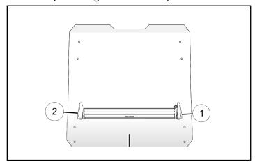
2. Line up center point of light bar assembly with center line of roof. Make sure that there is clearance underneath the roof for the fasteners and lightbar harness.
