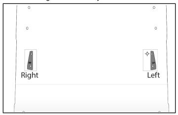
6. Mark all five holes on template as shown. Drill five holes as specified.
