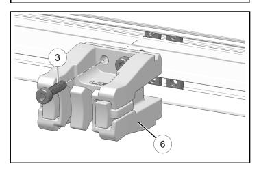
4. Move mounts according to distance, as shown below.
