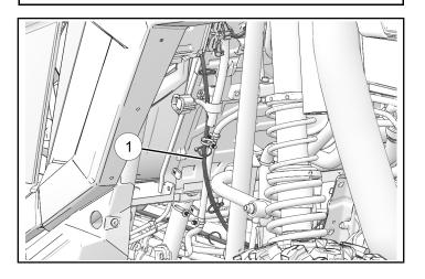
11. Route harness ① around chassis tube and top of shock.
