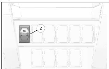
6. Locate vehicle power plug under dash. Remove cap from power plug.
