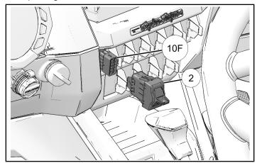
5. Push switch ② into dashboard until snaps into place.
