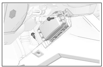
3. Install driver side panel with eight retained center console fasteners and one push-pin rivet. Torque fasteners to specification.
