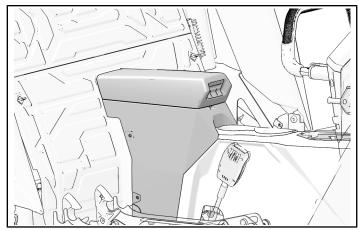
2. Install console storage compartment with two retained center console fasteners from passenger side. Torque fasteners to specification.
