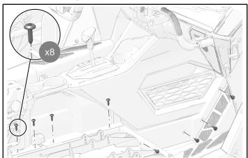
3. Remove and keep two push-pin rivets.
