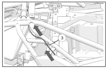
10. Connect chase light harness connector **6F** to chase light fixture.
