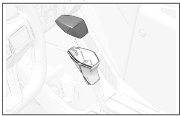
5. Remove and keep screw, pull shift knob from shift lever.
