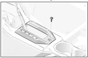
8. Carefully lift center panel upwards to remove side panels from vehicle.
