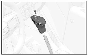
6. Lift and remove rubber trim piece from shifter gate opening to access screw.
