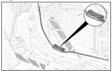
14. Examine harness routing and secure loose areas with cable ties ③.
