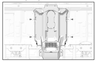
3. Remove and keep four push-pin rivets.
