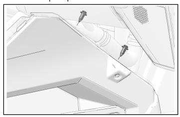
3. Install passenger side panel with eight retained center console fasteners and one push-pin rivet. Torque fasteners to specification.
