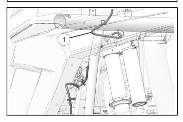
12. Route harness ① up through opening behind side panel. Attach to chassis using cable ties.
