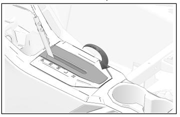
10. Install shifter knob onto shaft and attach with retained screw. Torque screw to specification.
