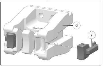
3. Align one mount **6** with four square nuts and install with four fasteners **3**).
