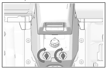
8. Install screw into shifter trim panel. Torque screw to specification.
