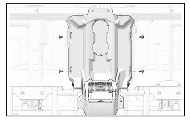
4. Attach to front-center console with two center console top fasteners (longer). Torque fasteners to specification.
