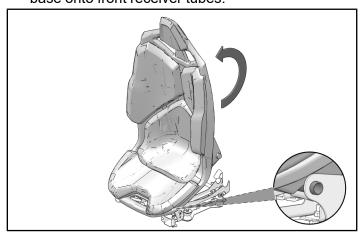
2. Lower seat onto rear receiver tubes.
