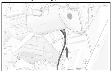
2. Install fuse block **F** to accessory mounting panel position 3, located in dashboard storage opening. Connect **3F** to Pulse® Bar.
