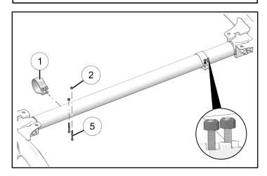
7. Align two mounts with clamps and install between clamp ends so that fasteners slide in between mount openings.
