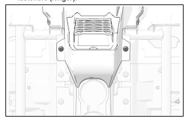
2. Remove and keep four center console side fasteners (shorter).
