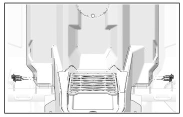
4. Lift rear center console and disconnect 12V outlet. Remove center console.
