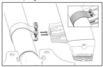
8. Tighten clamp fasteners 5 to specification.
