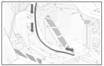
Multi-passenger vehicles only: Put harness down center of vehicle beneath rear seat panel.
