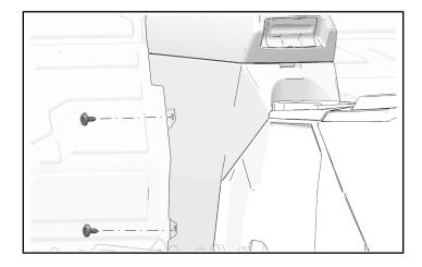
3. Install console storage compartment with two retained center console fasteners from driver side. Torque fasteners to specification.
