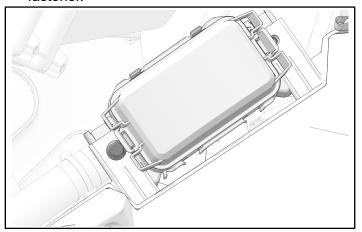
5. Turn fuse block upwards towards front of vehicle to access push-pin rivet beneath fuse block.
