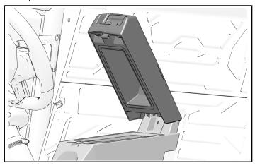
2. Turn each knob 1/4 turn to disengage from center console panel.
