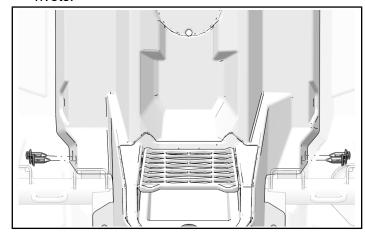
Install sides with four center console side fasteners (shorter). Torque fasteners to specification.
