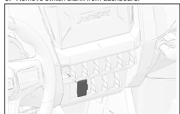
4. Put switch connector **10F** through dashboard opening and connector to switch ②.
