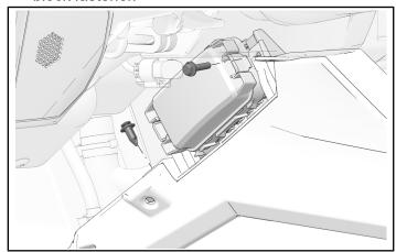
4. Loosen, but do not remove, left fuse block fastener.
