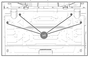
2. Turn two fasteners one quarter turn to disengage and remove bottom close-off panel.
