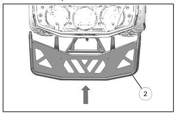
3. Loosely install two kept screws to attach rear rack extender to vehicle.
