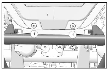
6. Loosely install two screws ③ in weldments ① to attach middle rack extender mounting tabs to frame. Torque four screws ③ to specification.
