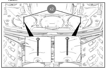
2. Put rear cargo rack extender on vehicle. Line up two top mounting tabs where screws were removed in Step 1.
