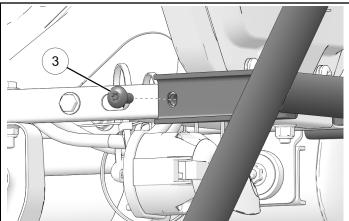
7. Torque two fasteners at top of rack to specification.
