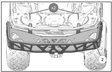
4. Put two weldments ① inside tube above rear hitch receiver. Loosely install two screws ③.
