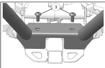
5. Put two weldments ① inside chassis tubes. Line up with middle rear rack extender mounting tabs.
