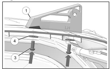
3. Torque screws on bracket from underside of roof panel.
