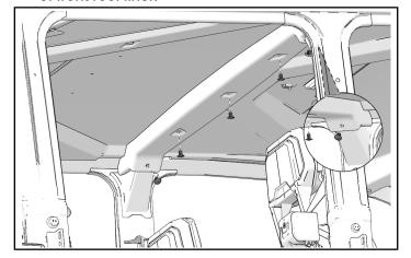
6. Three-passenger Model Only: Install two screws and two push dart clips from rear of front liner. Torque screws to specification.
