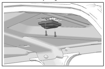
4. Crew Model Only: Remove five push dart clips from back of front roof liner.
