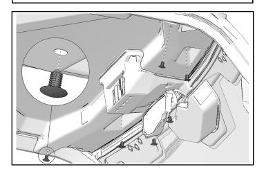
3. If vehicle is equipped with switch panel, install switch panel with two screws. Connect any wiring necessary. Torque screws to specification.
