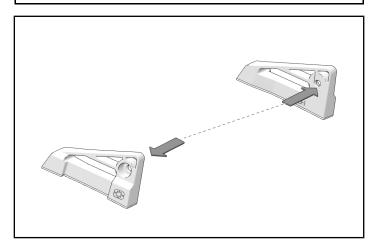
2. Measure length of light bar and bracket assembly to determine which set of pre marked holes to drill.
