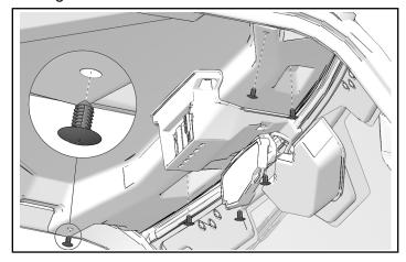
2. If equipped with upper switch panel, remove two screws from switch panel. Disconnect any harness attached. Remove Switch Panel.
