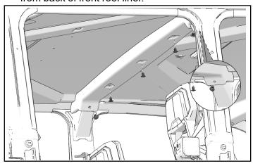
5. Three-passenger Vehicle Only: Remove two screws and two push dart clips from rear of front liner.
