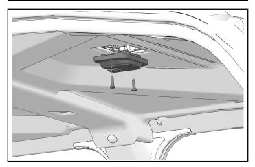
5. Crew Model Only: Install five push dart clips to rear of front roof liner.
