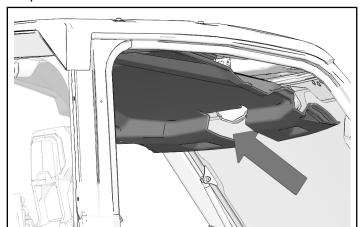
2. Install six push darts clips at front of roof liner.
