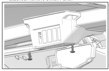
3. Remove two screws from middle of front roof liner. If equipped with dome light, remove dome light and disconnect any wiring.
