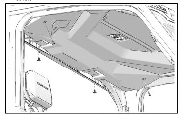
6. Pull front of roof liner down to remove from roof.
