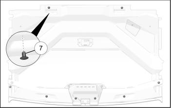
11. Loosely install two kept screws and washers to rear corner of headliner.
