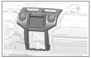
2. Attach upper center dash trim panel with four screws on top and two screws on lower edge of panel. Torque screws to specification.
