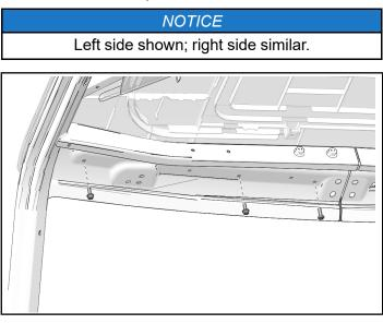
3. Slightly lift up roof edge and install visor seal ④ by tucking center of seal under roof edge and applying pressure starting with center moving outward.
