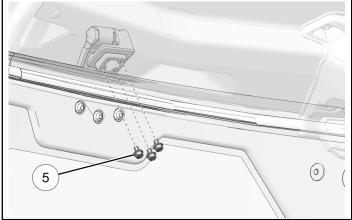
7. Torque screws (5) to specification.
