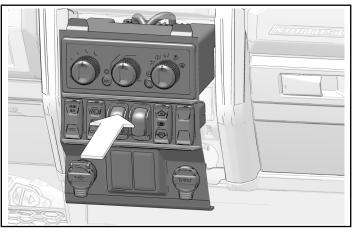
2. Attach with two push-pin rivets.
