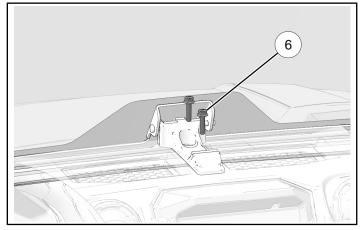
9. Torque two screws (6) to specification.
