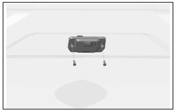
13. Torque two dome light screws to specification.
