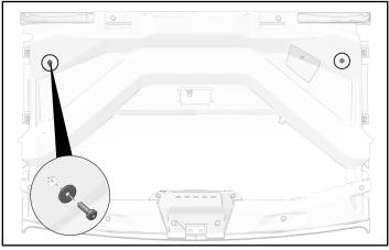
12. Connect dome light and loosely install using two kept screws.
