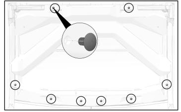
3. Remove headliner from roof and carefully set aside.
