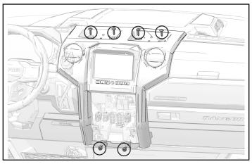
2. Lift upper center dash trim panel and disconnect any wire connectors. Remove upper center dash trim panel and carefully side aside.
