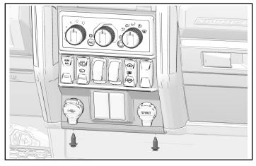
2. Remove center dash HVAC control panel trim and assembly. Disconnect any connections if needed.
