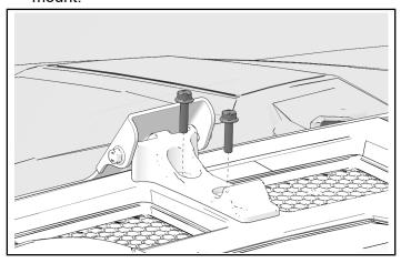
2. Remove and keep screw and nut from windshield (P/N 2889086) and remove windshield mount.
