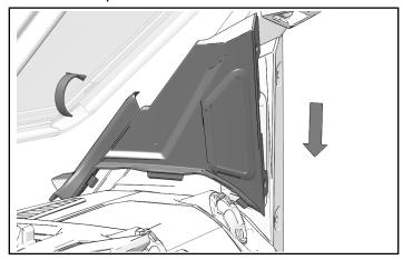
12. Install kept push-pin rivets in a-pillar panel.
