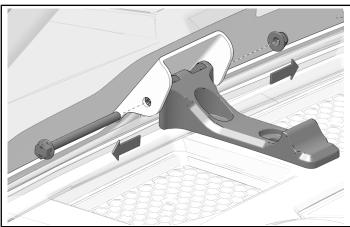
3. Install handle receiver ② using two screws ⑥.
