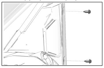
13. Loosely install upper ball end ④ to windshield bracket using nut ⑦.
