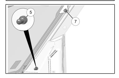
16. Install gas shock assembly ③ to ball ends.
