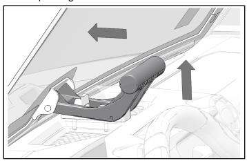
2. Push handle down into recession in handle receiver to lock in place.
