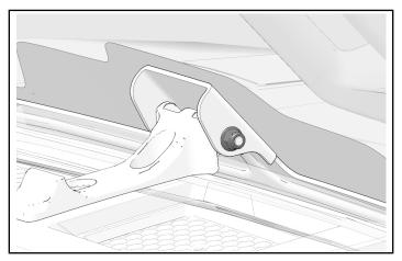
6. Remove and keep push-pin rivets from inner a-pillar panel.
