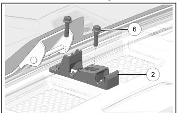
4. Install windshield handle assembly ① to windshield bracket with kept screw and nut.
