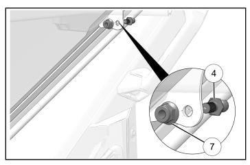
14. Loosely install lower ball end ⑤ to previously drilled hole in inner a-pillar panel.
