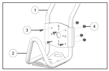
3. Align upper extension ① with tool holder by lining up the holes.
