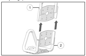
2. Attach upper extension ① to lower extension ② using screws ③ and nuts ④. Torque to specification.
