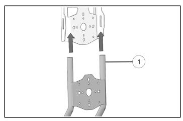
4. Attach upper extension ① to tool holder using screws ③ and nuts ④. Torque to specification.
