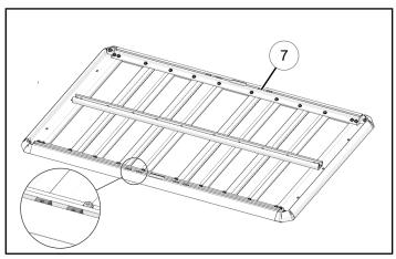
5. Install front ①,② and rear ③,④ braces on rack. Use two screws ⑨ to attach each brace. Tighten screws enough that braces do not slide when rack is flipped over.
