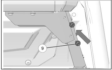
9. Torque screws (9) that hold braces to rack to specification. Use torque wrench to tighten screws.
