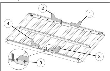
6. Flip rack over and place on backbones. Adjust rack to line up mounting holes with holes in backbones. Install six screws ③. Torque screws to specification. Use torque tool included with platform kit to tighten screws.
