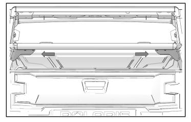
8. Install two screws (9) in each brace. Torque screws to specification. Use torque wrench to tighten screws.
