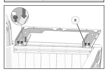
4. Turn bottom side of platform rack face up. Insert eight channel nuts ① through the large center slot into rack. Slide two channel nuts toward each corner of the rack.
