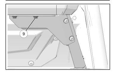
10. Torque eight screws ® that hold backbones to rails to specification.
