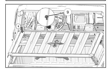
7. Slide front and rear braces out toward backbones until holes in braces line up with holes in backbones.
