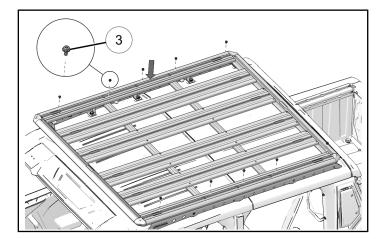
4. Adjust position of platform rack as needed. Torque screws ③ to specification. Use the torque tool that was provided with the platform rack.
