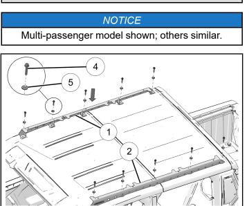
3. Install platform rack on the top of the backbones. Loosely install 10 screws ③.
