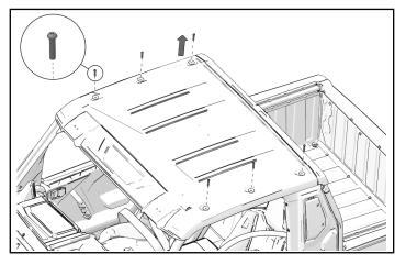
2. Install right ① and left ② backbones. Install screws ④ and washers ⑤. Make sure that the rubber side of the washers faces downward.
