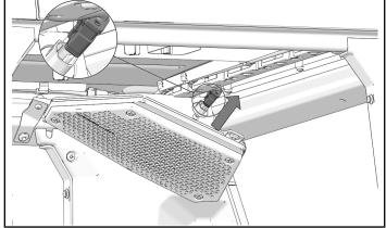
2. Remove and keep two screws. Remove the speaker.
